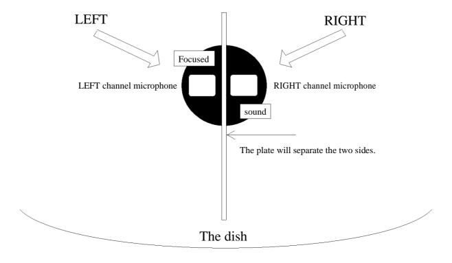
**STEREO MK3:** The plate separates the two sides from each other, while the focus from the dish will affect the two microphones equally **Result:** the focused sound will be presented in mono, while the background will be stereo, to L&R channels. NOT M/S! (3 channels)
